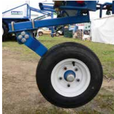
Rubber suspension elements for wheel suspensions on sprayers
