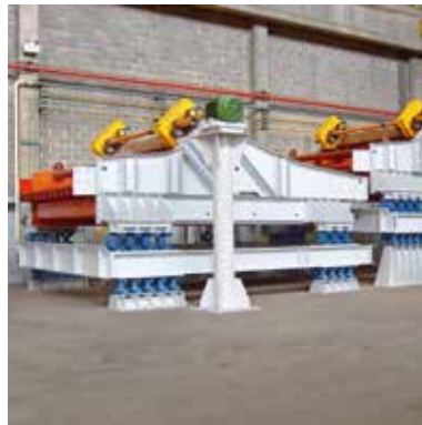
Oscillating mountings for isolating the base frame of vibrating screens
