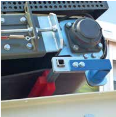
Tensioner device for conveyor belt scrapers
