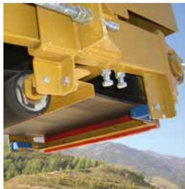
Tensioner devices on conveyor belts in the recycling sector
