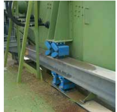
Counter-oscillating frame mounting for a vibrating screen
