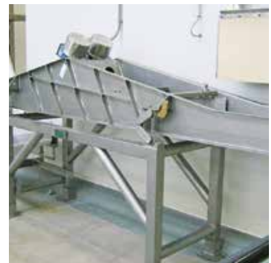
Dosing chute for vegetables on stainless steel ABI mountings
