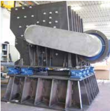
Vibration damper for recycling crushers
