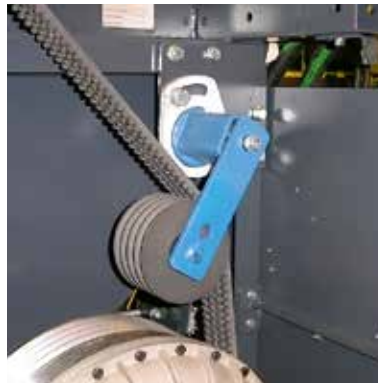
Tensioner device for belt drives in street sweepers
