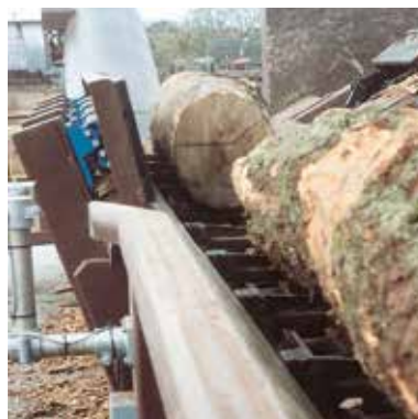
Dampening of an impact bed for logs
