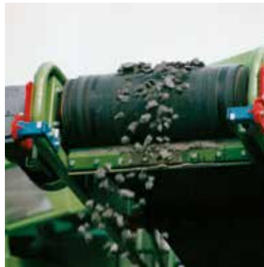
Suspension for belt scrapers on conveyor belts
