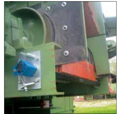
Rubber suspension element for conveyor belt scrapers
