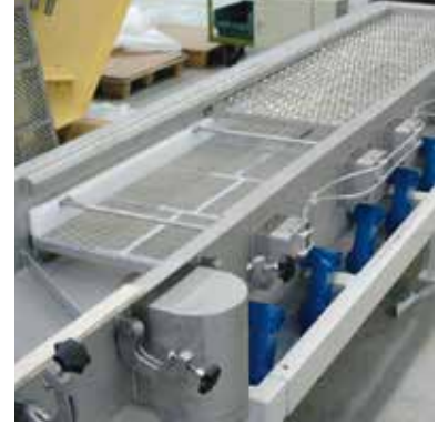
Oscillating mountings for sorting machines in the recycling sector
