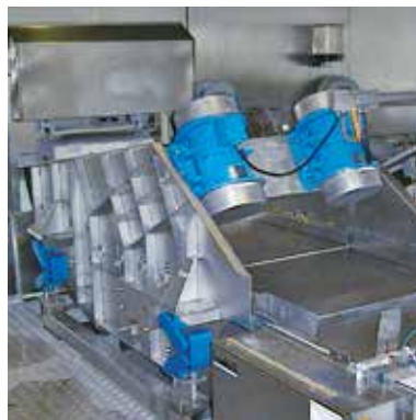
Washing and drainage screen for vegetables on AB mountings
