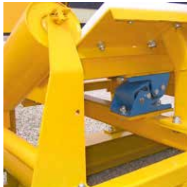
Vibration damper for the impact cradle
