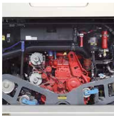
Tensioner devices for belt drives in buses
