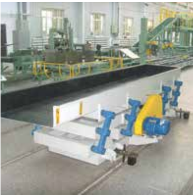
Two mass shaker for bulk solids with double rockers
