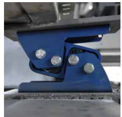
Cabin mounting with a vibration damper on a construction machine
