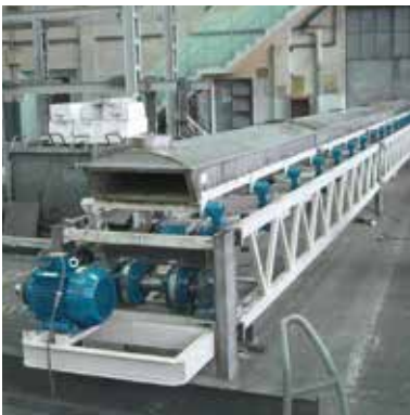
Two mass shaker for tobacco leaves with double rockers
