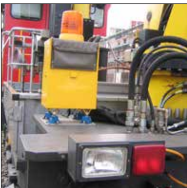
Vibration isolation for an electric cabinet on construction machinery
