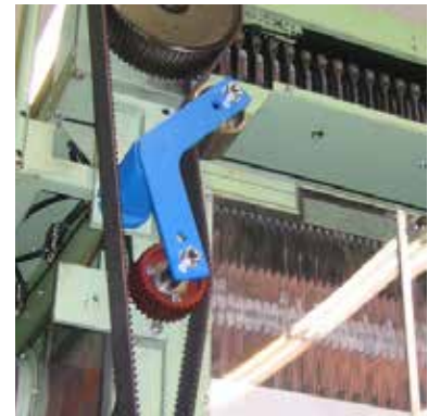
ROSTA Boomerang tensioner to tension long V-belts
