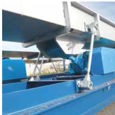
Conveying and screening chute for wood splinters
