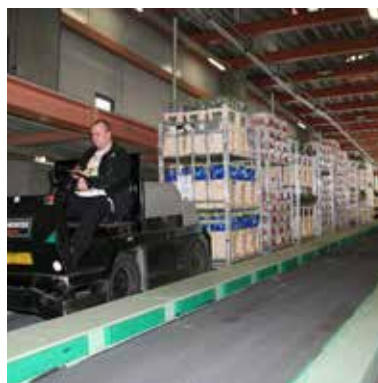
Vibration damper installed in the rail section as a side guide and break
