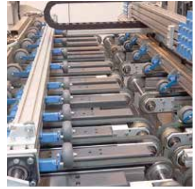
Tensioner devices as pusher units for transfer lines
