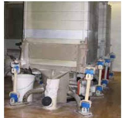
Vertical plane sifter with universal joints
